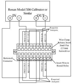
Figure 7.4: Analog Calibration Connections - Forward Voltage Channel
