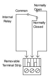
Figure 5.9: Relay Output Connector
