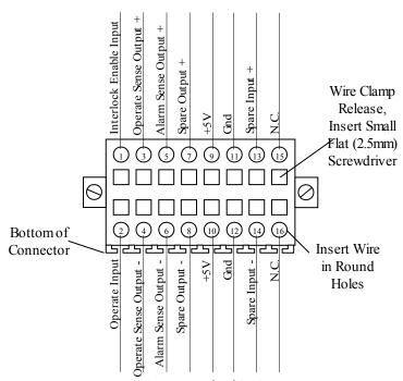
Figure 5.6: Digital I/O Connector
