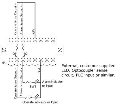
Figure 5.8: Digital Output Connections
