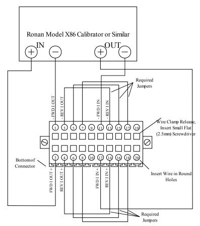
Figure 7.2: Analog Calibration Connections - Forward Current Channel
