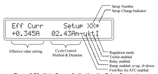
Figure 6.29: Main Screen Indicating the Setup Parameters
