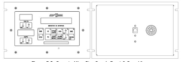
Figure 5.3: Remote MicroStar Panel: Front & Rear Views
