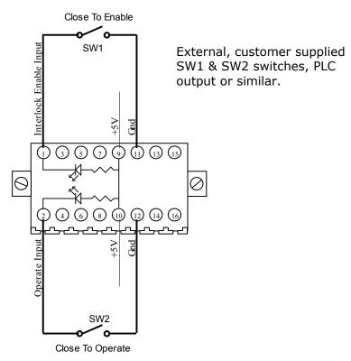
Figure 5.7: Digital Input Connections
