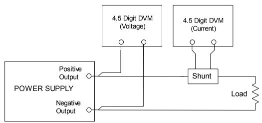
Figure 7.1: Output Calibration Connections
