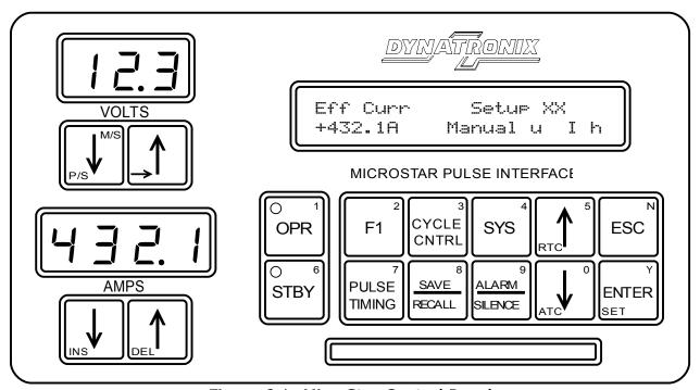
Figure 6.1: MicroStar Control Panel
