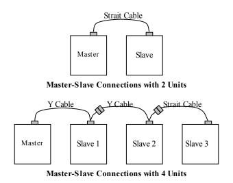
Figure 5.12: Connection Diagrams for Single and Multiple Slave Units
