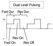
Figure 6.25: Dual Level Pulsing Example
