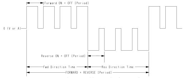
Figure 9.3: Three Possible Periods of a Waveform
