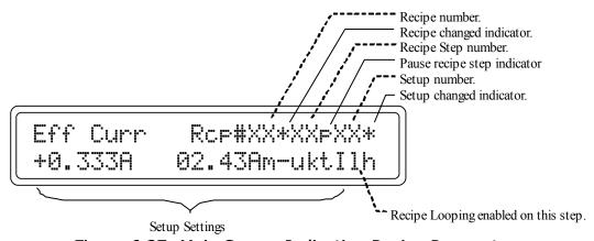
Figure 6.37: Main Screen Indicating Recipe Parameters
