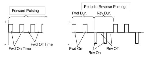
Figure 6.24: Pulse Timing Examples
