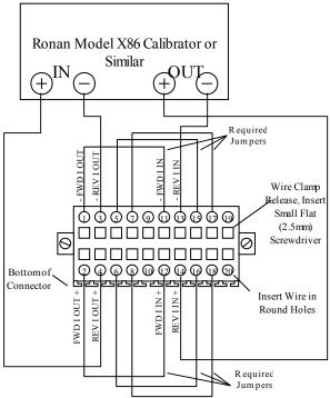
Figure 7.3: Analog Calibration Connections - Reverse Current Channel - (option)
