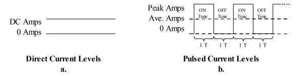
Figure 9.1: DC versus Pulse Currents
