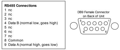
Figure 5.4: RS485 Wiring Connections
